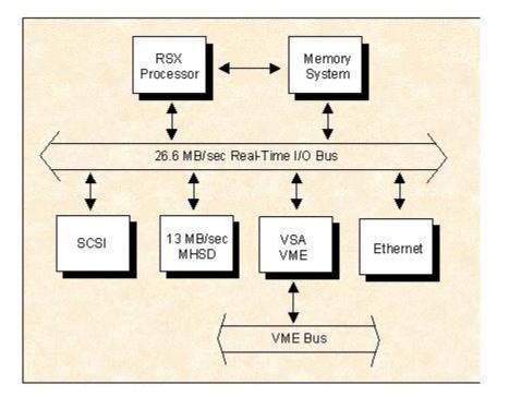
Figure 3. Real-Time I/O Bus Copyright © 2020 Compro Computer Services, Inc. All rights reserved.
