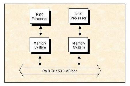
Figure 4. Integrated Multi-CPU Cache Coherency
